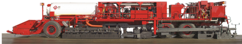
Receiving Hopper for New HMA
